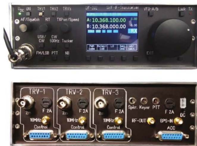
PHOTO 1: Prototype 144MHz SDR from DK2FD and DF0MU (thanks to them for the photo).
