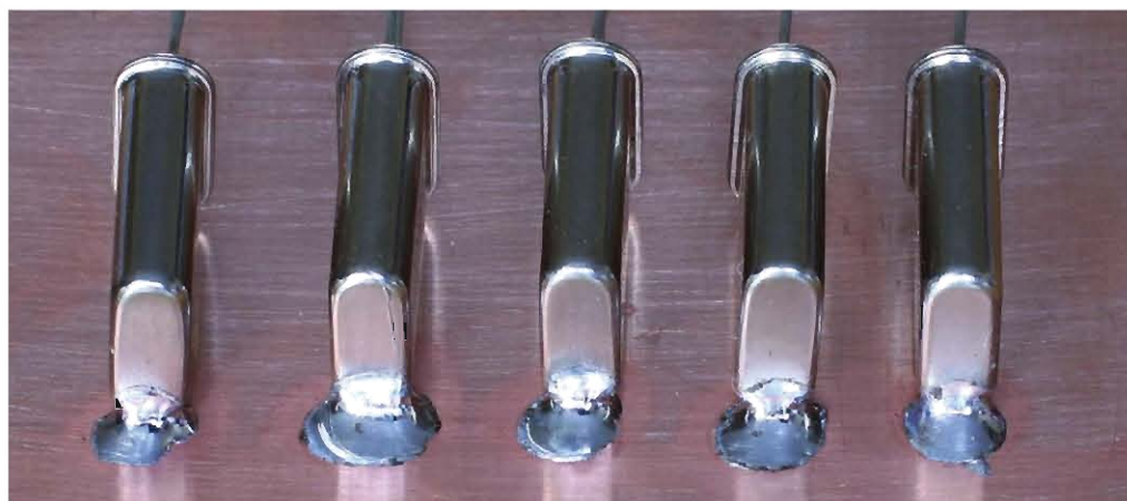
PHOTO 3: Soldering crystal cans to the PCB makes for a firm mounting.
