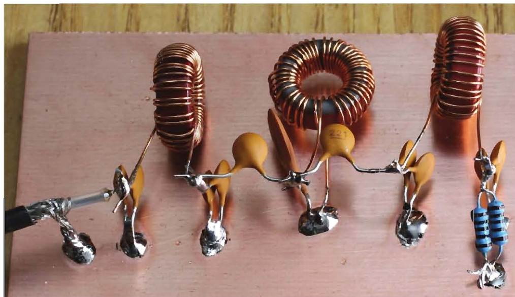
PHOTO 2: Completed prototype 160m bandpass filter.
