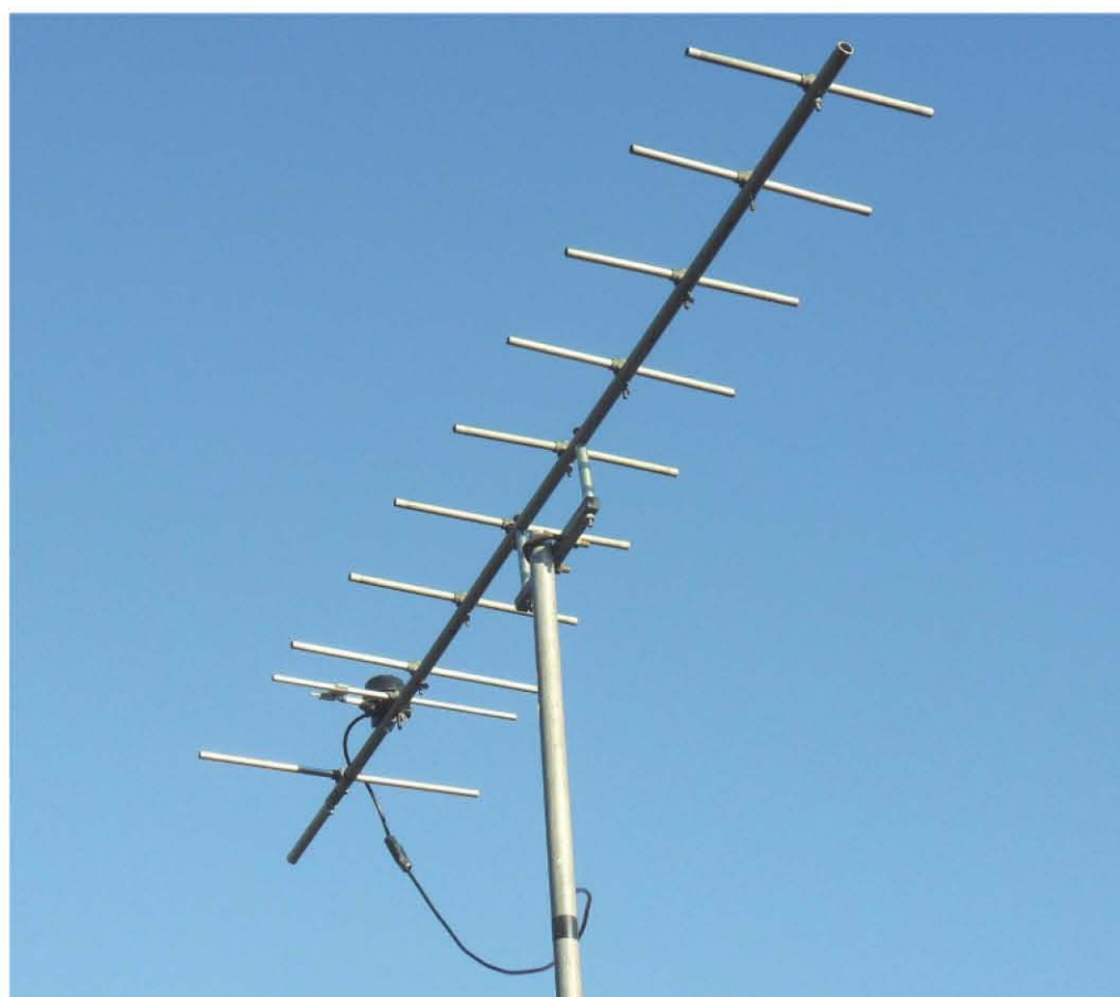
PHOTO 5: The gamma match in use on the 10 element Yagi beam.
