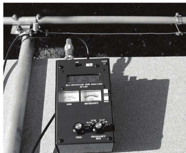
PHOTO 1: G3LDO's HF gamma match under test.
