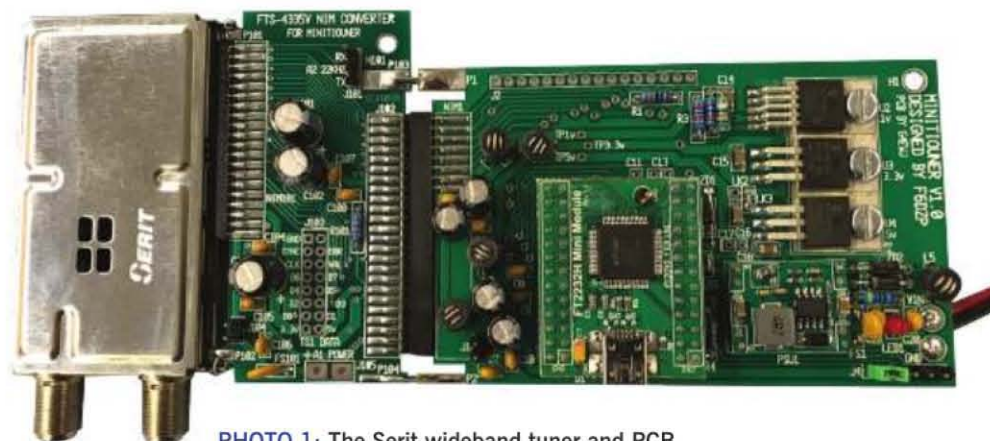
PHOTO 1: The Serit wideband tuner and PCB.
